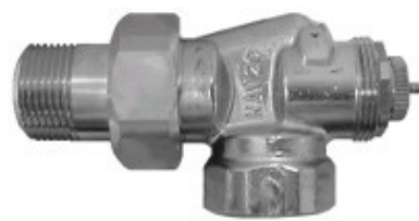
Horizontal angle valve with straight nipple. NPT - female inlet, male union outlet. 1/2" - N10837 3/4" - N10857 1" - N10877 1-1/4" - N10897
