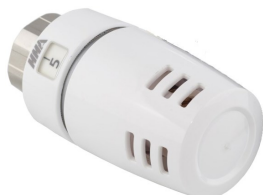
EVO - Non-Electric direct mounting thermostat with a numerical window reading that corresponds to various temperatures. May be limited or locked if required. Features heat diffusing rings to dissipate heat away from sensor for added accuracy.
