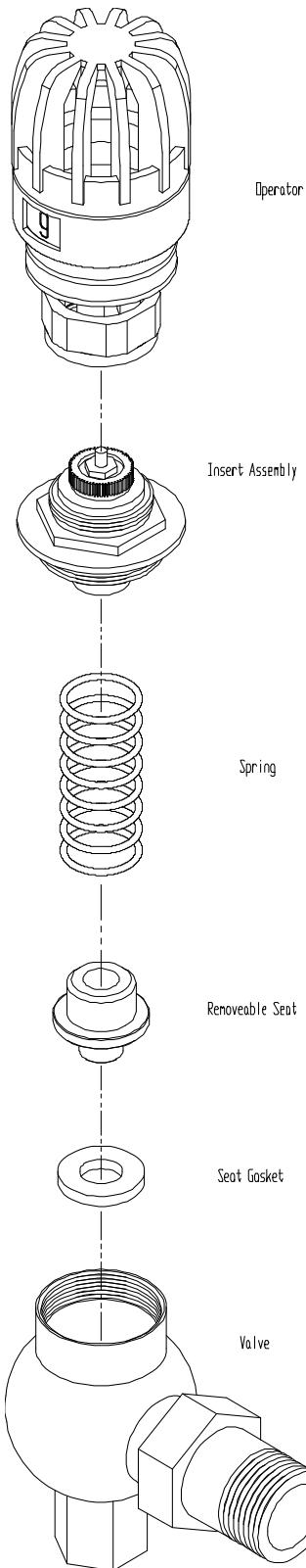
1. Remove existing valve components. Thoroughly clean and inspect interior of valve.
