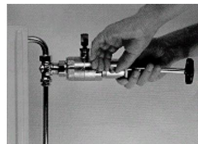
6. Open the drain cock to relieve water or steam pressure in the chamber.
