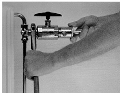
2. Place the socket of the insert changer onto the valve insert. Press in the stem handle of the tool to ensure a firm engagement.
