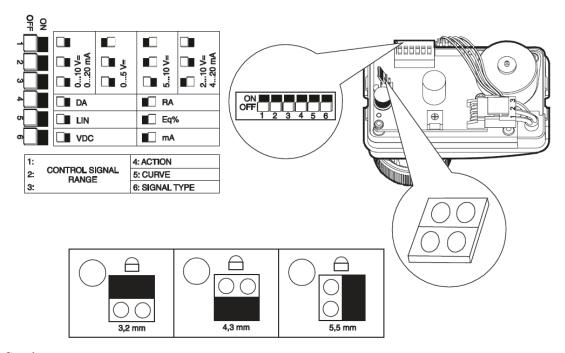
Factory Setting: All the DIP switches in OFF position.
